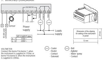
Note: The length of the cable for the sensor may be increased by the user up to 200 meters, using PP2x24AWG cable. For immersion in water use thermometric well.
